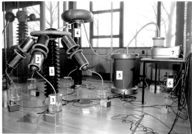
Figure A2. The PD test set-up. The numbers refer to the list of components on the preceding page. Top: diagram, bottom: photo of the set-up.
